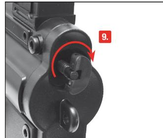
9. Tighten cylinder retention screw, pierce CO<sub>2</sub> cylinder.
