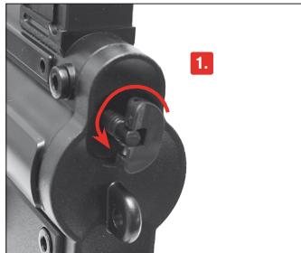
1. Unscrew cylinder retention screw.
