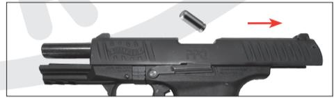
Remove the magazine. Remove cartridge from the barrel by pulling back the slide.
