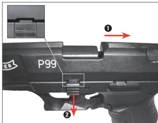
Cock internal hammer by pulling the slide back.
