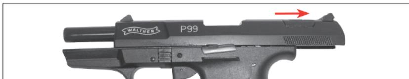
Pull back the slide and allow it to spring forward. This transports the cartridge to the barrel. The gun is now loaded.
