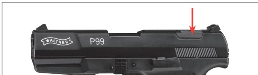
To decock the gun, press the decocking lever. The hammer will audibly decock.
